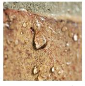
Watco Masonry Waterproofer penetrates deeply over time, so it can take up to two months for a noticeable beading effect to appear when rain strikes the wall. Curing times will vary depending on the porosity of the surface and weather conditions.
